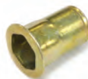
Hex Body threaded insert for punched holes provides exceptional spin out resistance. Available in steel, brass and 302 stainless steel.
