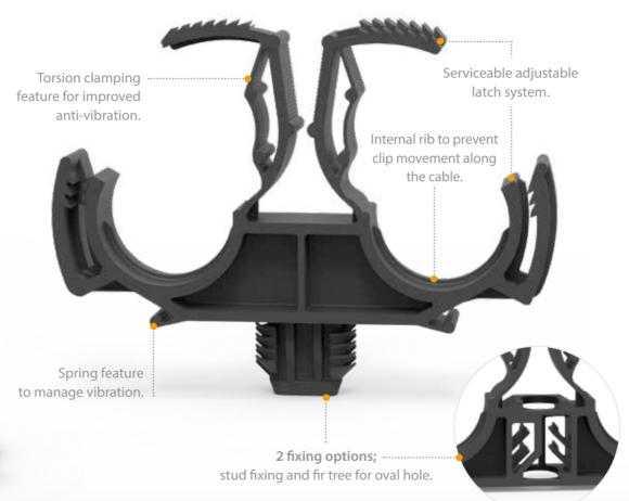
Manage a wide range of applications due to multiple diameters, oval hole or stud fixing, single or double cable housing.
